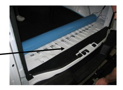
After plastic trim is cut and back in it's original location, you must measure 7" inches forward on both sides from newly cut trim to place rear Kwik Kit bulkhead.
